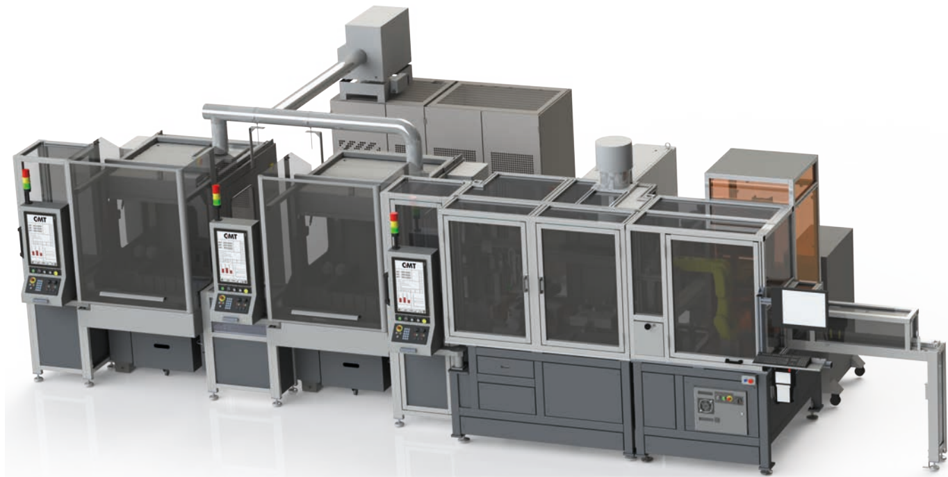
The picture shown is a production line to grind the groove and profile form in turbo charger shafts
